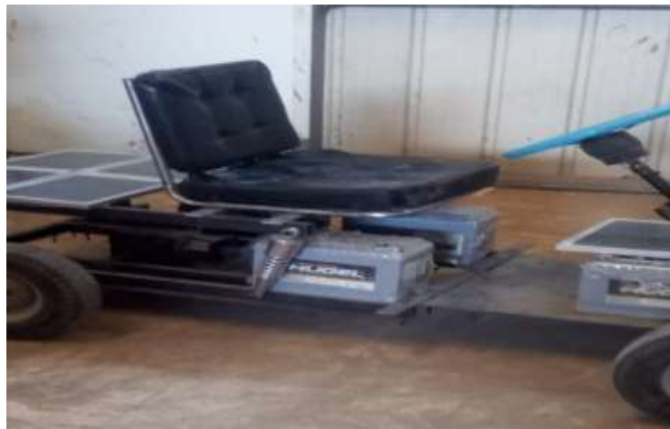
Fig. 3.2 b: Experimental prototype using PV solar of electric vehicle.
