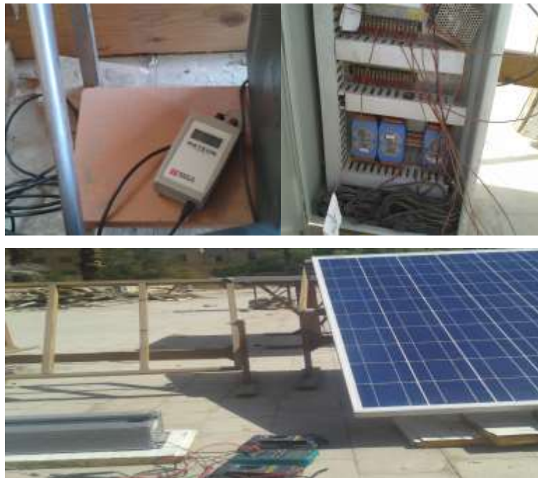
Fig. 3.2 a: as shown the measurement devices such as solar radiation, temperature measurement, variable resistance, and PV module
