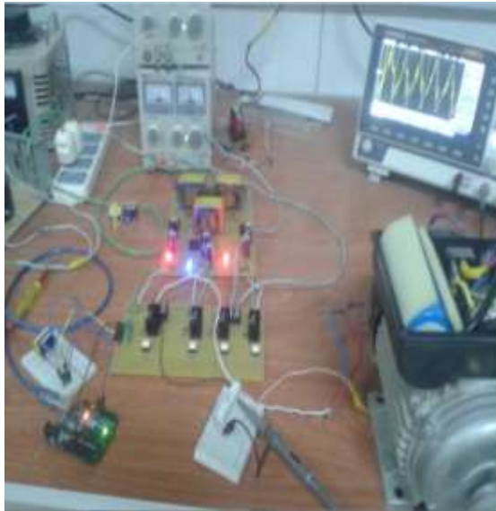
Fig. 4.23: A picture for the experimental prototype single phase inverter
